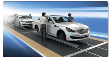
The Skid Transfer System
