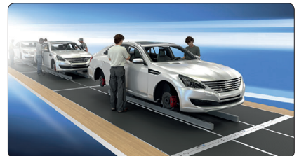
The Skid Transfer System
